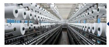
Cone Winding: Final stage where yarn is wound into cones so that it can be shipped to the customer.
