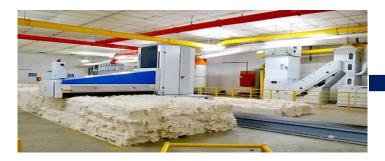
Blow Room: the compressed bales are opened, cleaned and blended/mixed according to particular length to form a specific size of lap.
