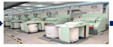
**Carding:** The lap is shifted to carding machine where cleaning and intermixing of fibers occurs to produce a continuous web.
