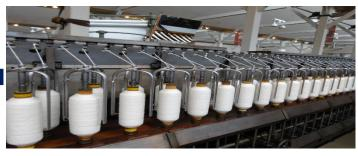
**Roving/Ring Frame:** Roving frames carry out process of converting fibers into low twist lea. Further twisting is done to form yarn of required count and strength.
