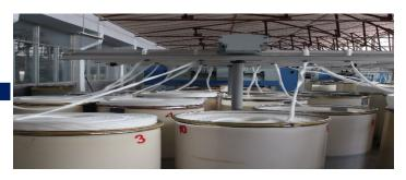
**Drawing:** Strengthening of fibers by passing them through rollers.
