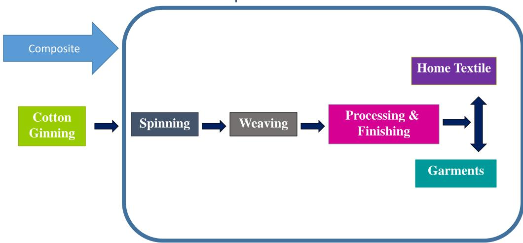
Composite Textile unit includes all processes from spinning of yarn to finished good
