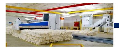
**Blow Room:** the compressed bales are opened, cleaned and blended/mixed according to particular length to form a specific size of lap.
