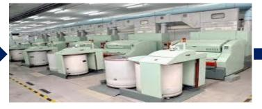
**Carding:** The lap is shifted to carding machine where cleaning and intermixing of fibers occurs to produce a continuous web.
