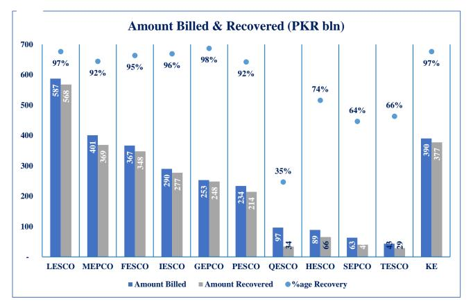
Other than distribution line losses, non-recovery of billed amounts from consumers for the DISCOs in the CPPA-G system stood at ~9% and at ~3% for KE in FY22. The cumulative cost of non-recovery stood at PKR~243bln.
